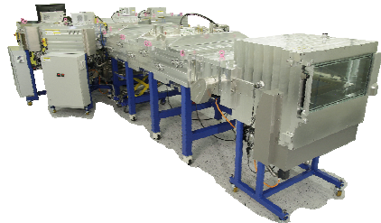
PECVD and PVD for complete SHJ deposition cycle
